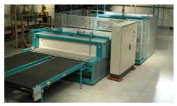
This option avoids to change the film roll to adapt width and thus saves time. The shrinkwrapping process is optimized and requires less plastic film (less waste).
