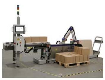
Designed to be easy to use, intall and set up, CoboAccess\_Pal can be quickly moved by the operator on another line thanks to outstanding Plug and Play features. Easy to move and adapt, it can effortlessly be carried from one line to another using a forklift.
