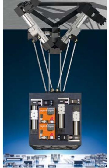
tems such as the robolink range. User can build customized robotic arms up to 5 axes from a modular system, using different joints associated with different plastic reducers, motors and linking components.
