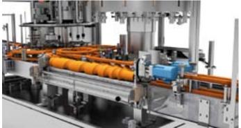
The machine still uses the weight-filling technology, known for its precision, reliability and cleanliness. Dosing cleanliness is further improved by using an analog probe which ensures real-time monitoring and filling of the tank in order to optimize the gravity flow.
