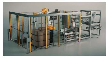
the positioning of the piles on the pallet. The layout of the cells is custom-made by TEC-MA-ARIES according to available space.
